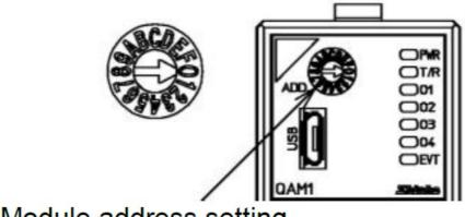
Module address setting rotary switch
