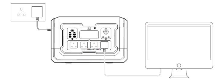
The product supports UPS to <20ms switchover time. When connected to grid power, activate the AC on the unit and use your appliances via the front sockets (AC power will come from the grid and not the BASE 2.5 power unit in this case). In case of a grid failure, the unit will automatically switch to the battery powered AC supply mode within 20 milliseconds.
