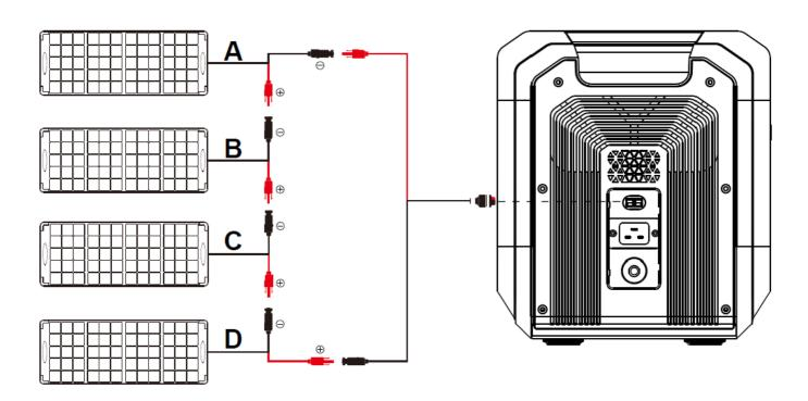
Connect the solar panels to the Anderson input on the side of the unit by using the supplied Anderson to MC4 cable. Multiple solar panels can be connected in series or parallel to achieve the desired input (which should be within the specified 12-150V range). Maximum power input is 2100W, which will charge the unit in one hour.
