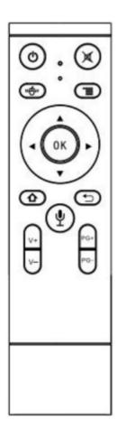
Bluetooth connection mode After the remote control is powered on, press the Key + key at the same time to turn on the Bluetooth connection mode. At this time, the indicator light flashes slowly. The device searches for the Bluetooth name "Bluetooth remote". After clicking the connection success, the indicator light goes out.
