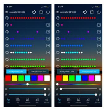
• **Rbm Mode** 100 patterns of change, slide the ring to select pattern effect, and slide "a" or "I" for overall pattern effect brightness or speed settings. Click on "AUTO" to enter cycle mode or click on the heart icon to mark the favorite effect.
