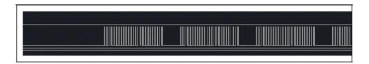
1. The code has 24 bits in total, BYTE0+BYTE1+BYTE2+end bit BYTE0, BYTE1 is the address code, the address
