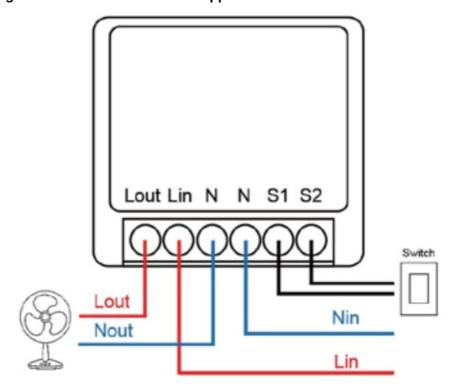
4.2 The wiring diagram to connect the light.
