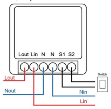
Warning: S1 and S2 can only be connected to the two ends of the wall, and cannot be connected to strong power such as a zero-fire line.
