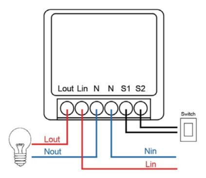
Power on after completion of wiring and the device is turned on by default, press and hold the button for about 5s seconds until the WiFil blue LED blinks fast.
