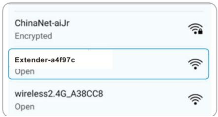
Connect to the extender network: Extender-a4f97c (The SSID on the label of the router) U9
