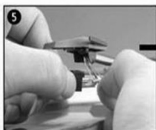
1 push the arm lock to release the tone-arm.
