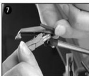
3 separate the cartridge from the socket lightly.
