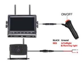
The monitor also can be powered by ACC / Fuse/ Radio etc.
