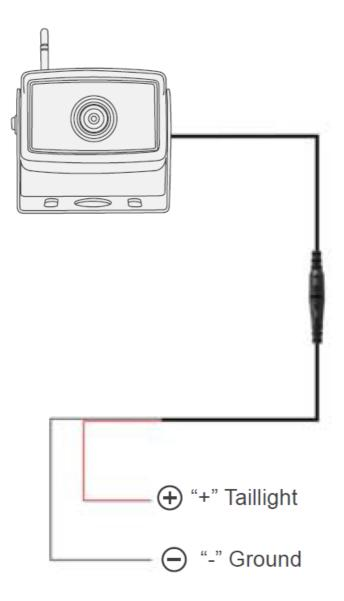
**Note:** Of connecting power directly to a battery, the cameras are always ON and therefore drain the battery. Therefore it is recommended to connect power to an ignition switched accessory power source.
