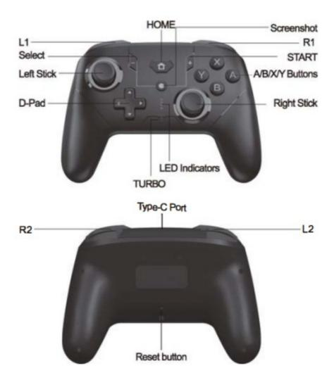
**Reset button function:** When the controller is out of order, which can be reset by poking the reset key at the back of it
