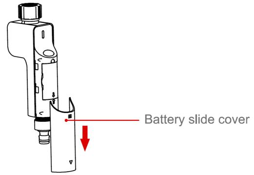
2. Remove the battery compartment.
