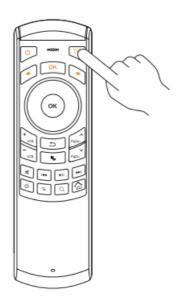
2. Align the original IR remote lamp with the air mouse keyboard IR lamp at a distance of 2-7cm and short press the corresponding button within 10 seconds. If the programming is made successfully. LED light blinks for 2 seconds and exits programming status. You can check whether the programming is successful. If not please repeat the above operation.
