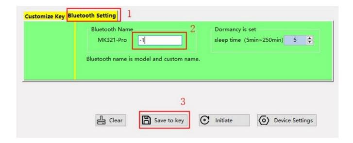
**Sleep time:** Click Bluetooth Settings, and you can set the sleep time in the input box of sleep time. The sleep time indicates how long the device will enter the sleep state after no action (without pressing the button).
