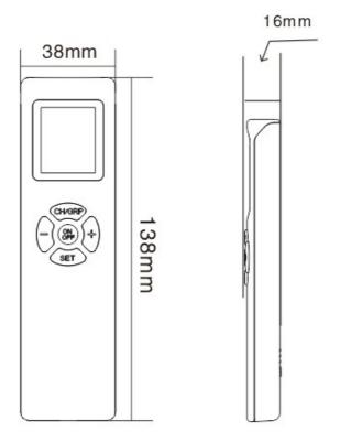
Unit: mm Tolerance: ±1.0mm L=138 W=38 H=16
