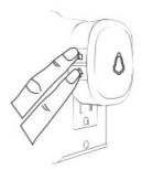
3. Short press the button to pair and trigger a transmitter to send a signal to the doorbell receiver. And you will hear and see:
