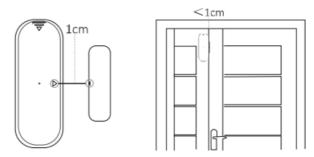
3. Fixing with double-side adhesive The surface (door or window) where the detector is to be installed must be clean and dry in order to ensure that the double-sided tape supplied adheres properly.
