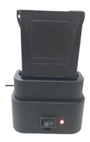
Put the device on the "Config&Recharge BOX", switch to recharge status, the "Config&Recharge BOX" the other side connects to the adapter, then red LED will be light.
