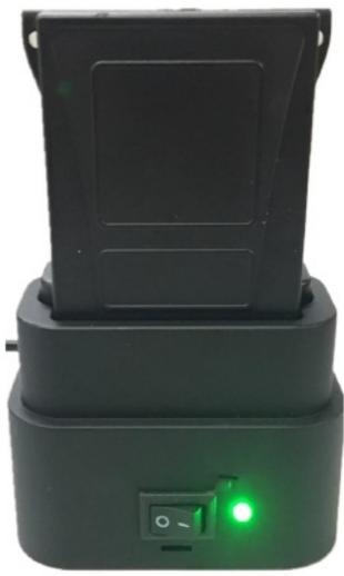
Put the device on the "Config&Recharge BOX", switch to config status, the "Config&Recharge BOX" the other side connect to computer, then the green LED will be light.
