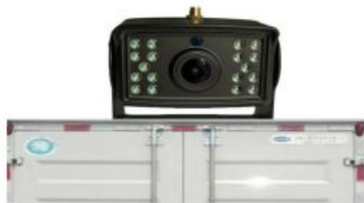
step1: Fix the camera on the container of truck with screws
