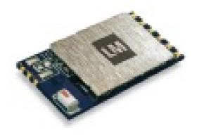
The product described in this document is the basic information of network module hardware, and the unified model name of network module is AZ820-HN. This module mainly establishes the network foundation for the large screen customer environment of commercial display. The products respectively support wired and wireless wan to realize data access to the external network, and provide high-speed and stable wireless hot spots to meet the terminal wireless internet access and business needs.
