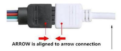
First connect the load line, then connect the power line; Before power-on, ensure that there is no short circuit between cables. When operating, the remote control points to the infrared receiving head to ensure that there are no obstacles between the remote control and the receiving head;
