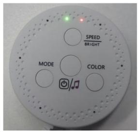
Red indicator light: when the indicator light is on, it indicates the energized state of the equipment. Green indicator light; Infrared indicator light, the remote control press the green light once and it will flash, indicating that the infrared signal is received. When the remote control has no operation, the indicator light is not on.
