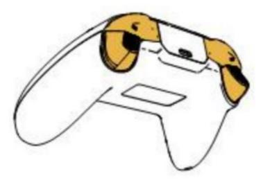
2. Hold LB, RT (or RB, LT) to return the robot to docking station
