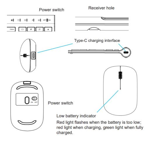
OAfter the keyboard is powered on, the green light will turn on for 3S and then turn off
