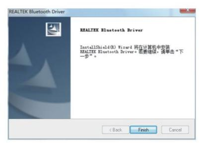
2. After the Bluetooth driver finishes installing, the task bar has a Bluetooth signal icon, click on the "add equipment"; and open your phone, PC will search Bluetooth information of the mobile phone. Click-Nexr, mobile will receive the verification code from PC that matches mobile phone with computer, PC click "Next, you could use normally with the Bluetooth function.
