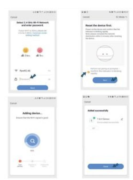
3) If your Wi-Fi router opens both 2.4GHz and 5GHz with the same name, enter a Wi-Fi password, please select "AP Mode", hold the reset button for about 5 seconds till the LED indicator blink slowly, connect your mobile to the device's hotspot: "SmartLife-XXXX", then click to return to App interface, it will connect to Wi-Fi automatically, configuration complete.
