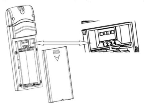
2. Before inserting the batteries, find the dip switches instruction above the battery compartment and set the following configuration:
