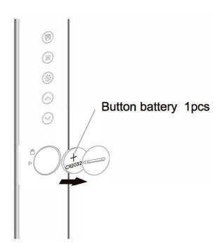
Before you change the battery press the battery case and push down it Then inserts 1pcs new battery and closes the battery case into the right position
