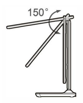
• Lamp head can be fold-able to 150' angle (It may be broken if you over-adjust)
