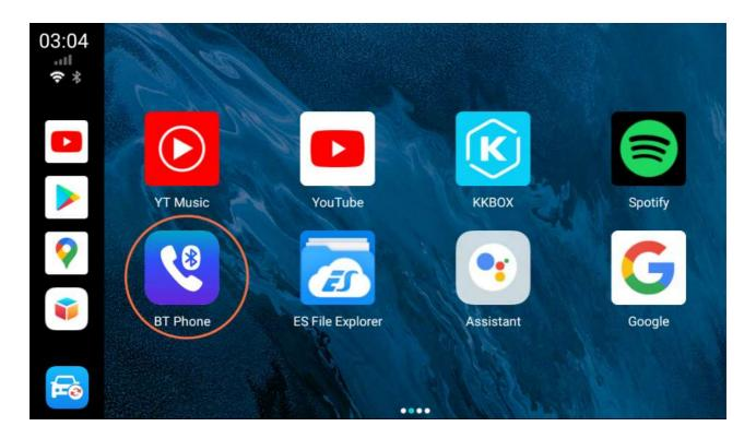
Search the mobile phone, Click to select the mobile phone to be connected, Click the pairing connection button to complete the pairing and connection
