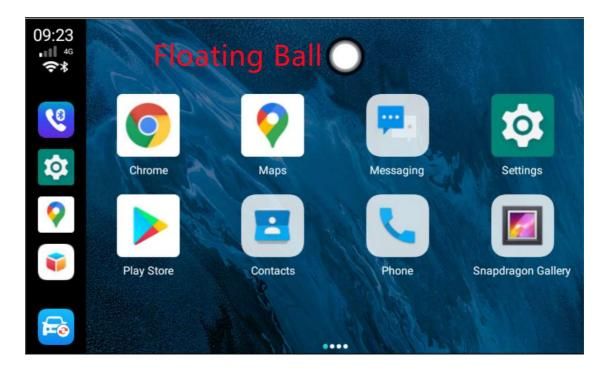
The functions of the row of buttons after clicking on the floating ball to expand are: Home, Return, Recently, Voice, Return to the original car UI, Clear memory and one button split screen display
