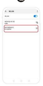
02. Open the phone system settings,Connect mobile phone Wi-Fi to "MV"At the beginning of the network, then open the APP
