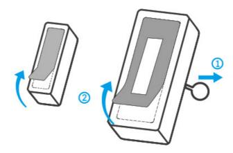
2. Try to align the marked line on the magnet with that on the transmitter during installation.
