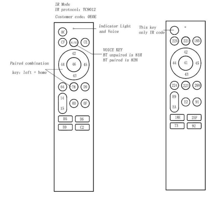
The remote control has two modes: infrared and Bluetooth.
