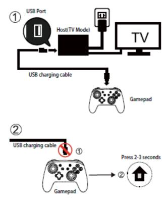
**Note:** When the handle has been paired with the host, short press the home button to wake up the host when it is turned off.
