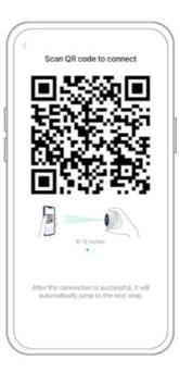
2. After pressing the camera switch for 3 seconds, the camera will turn on. At this moment, target the camera at the QR code of the mobile App, with a distance of about 20cm (about 7 inches) until the camera emits a "Di" sound, which represents the scanning is succeeded and the pairing is started.
