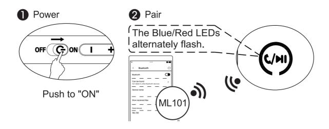
Long press the button for 2 seconds to enter pairing mode. (On first use, the ML101 will enter pairing mode automatically) The blue and red LED will flash.
