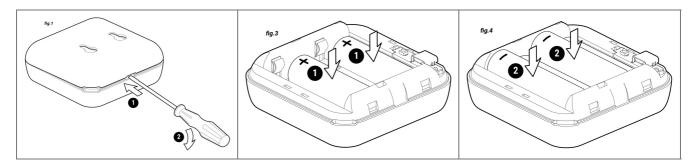
$\triangle$  CAUTION! Make sure the batteries + and – signs correspond to marking on the Device battery compartment (fig. 2 A)
