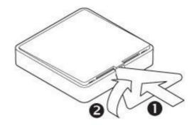
2. Extract the exhausted battery by first pushing it through the battery holder cutout and then pulling it out.
