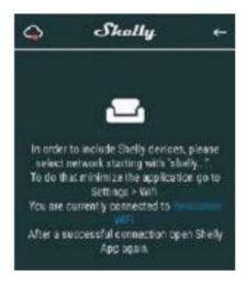
Press the home button of your iPhone/iPad/iPod. Open Settings > WiFi and connect to the WiFi network created by Shelly, e.g. shellyrgbw2-35FA58.. If using Android your phone/tablet will automatically scan and include all new Shelly Devices in the WiFi network that you are connected to.
