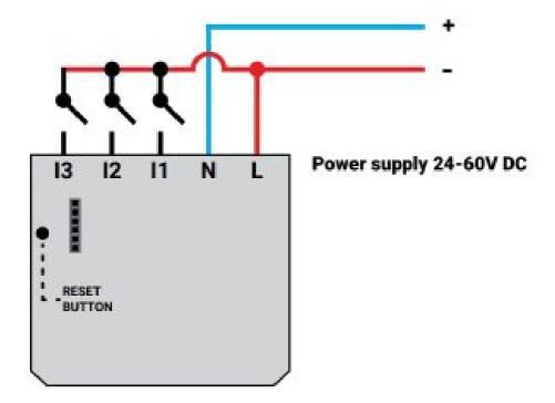
The WiFi switch input Shelly i3 may send commands for control of other devices, over the Internet. It is intended to be mounted into a standard in-wall console, behind power sockets and light switches or other places with limited space. Shelly may work as a standalone Device or as an accessory to another home automation controller.
