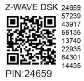
The first five digits of the key are highlighted or underlined to help the user identify the PIN Code part of the DSK text. The DSK is additionally represented with a QR Code as shown on the image.
