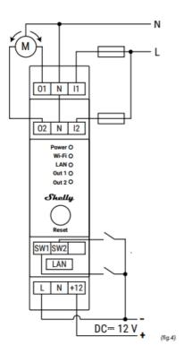
CAUTION! Do not connect the Negative wire to the N terminal, which is between the L and +12 terminals. Connect the common motor terminal/wire to the Neutral wire. Connect motor direction terminals/wires to the O1 and O2 terminals\*\*.
