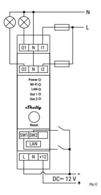
CAUTION! Do not connect the Negative wire to the N terminal, which is between the L and +12 terminals. Connect the first load circuit to the O1 terminal and the Neutral wire. Connect the I1 terminal to the first load circuit breaker. Connect the second load circuit to the O2 terminal and the Neutral wire. Connect the I2 terminal to the second load circuit breaker.
