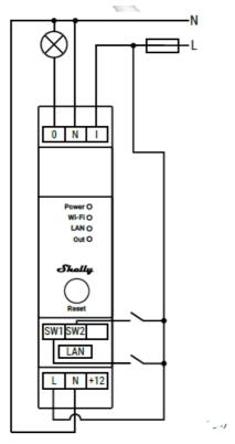
connect both N terminals to the Neutral wire and the L terminal to the circuit breaker. Connect the 2 switch circuits to the S1 and S2 input terminals and the circuit breaker. Connect the load circuit to the O terminal and the Neutral wire. Connect the I terminal to the circuit breaker.
