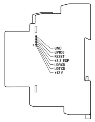
**CAUTION!** High voltage on the add-on interface when the Device is powered!
