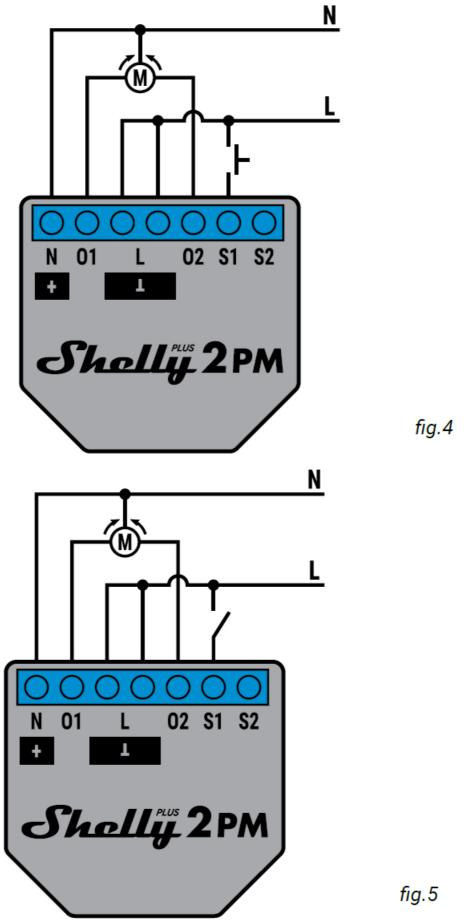
If the input is configured as a switch, each switch toggle cycles open, stop, close, stop...
