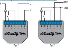
Connecting to the power grid with power supply 110-240 V AC (fig. 1), or 24-30 V DC\* (fig.2).
