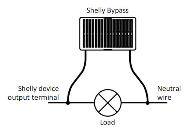
Connect the Shelly Bypass in parallel to the load as shown on the diagram above.
