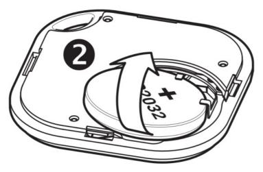
3. Slide in a new battery as shown on Fig. 2(3).
