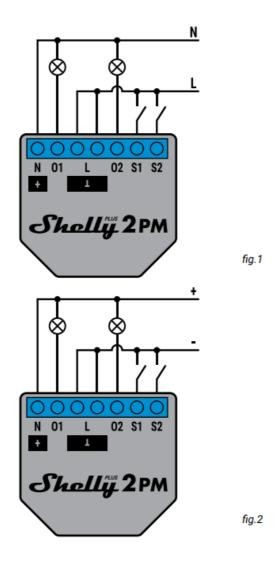
**CAUTION!** Use the same power supply for the two load circuits and the Device.
