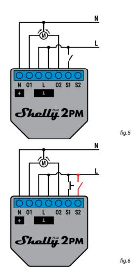
Connect the button or the switch to the S1 or the S2 terminal and the Live wire. If the input is configured as a button in the Device settings, each button press cycles open, stop, close, stop, etc.
