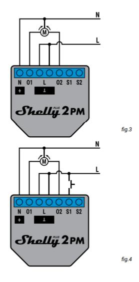
If you want to use the Device in single input mode connect the device as shown on Fig. 4 for a button input or Fig. 5 for a switch input. Connect both L terminals to the Live wire and the N terminal to the Neutral wire. Connect the common motor terminal/wire to the Neutral wire. Connect motor direction terminals/wires to the O1 and O2 terminals\*.
