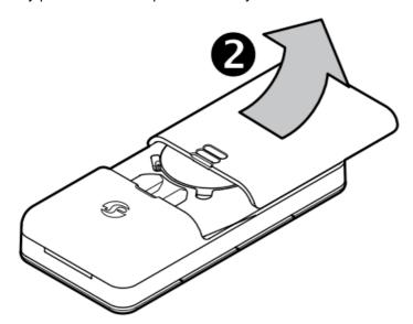
3. Remove the exhausted battery.
