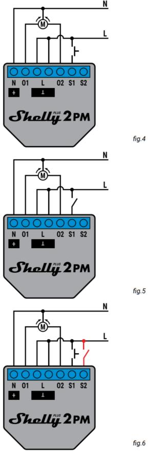
**△CAUTION!** Use the same power supply for the two load circuits and the Device.
