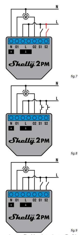
To utilize it, connect the device as shown on Fig. 6 for a button input or Fig. 7 for a switch input. Con- nect both L terminals to the Live cable and the N terminal to the Neutral cable. Connect the common motor terminal/cable to the Neutral cable.
