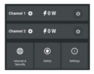
Safety – Max Power: You can limit the maximum power the socket will supply. If the pre-set current draw is exceeded, Shelly will turn the socket off. Allowable power can be set between 1 to 2300W.
