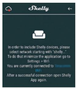
Press the home button of your iPhone/iPad/iPod. Open Settings > WiFi and connect to the WiFi network created by Shelly, e.g. shellyswitch25-35FA58. If using Android your phone/tablet will automatically scan and include all new Shelly Devices in the WiFi network that you are connected to.
