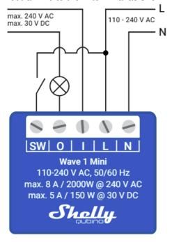
"Connect a switch or a push-button to the Device SW terminal and the Live wire.
